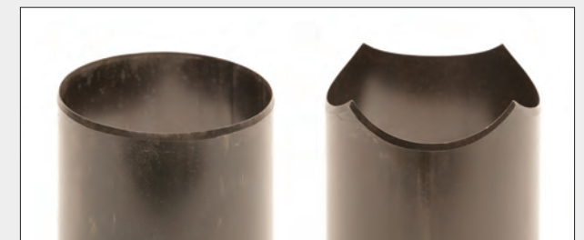
Outside sharpened: push up native soil
